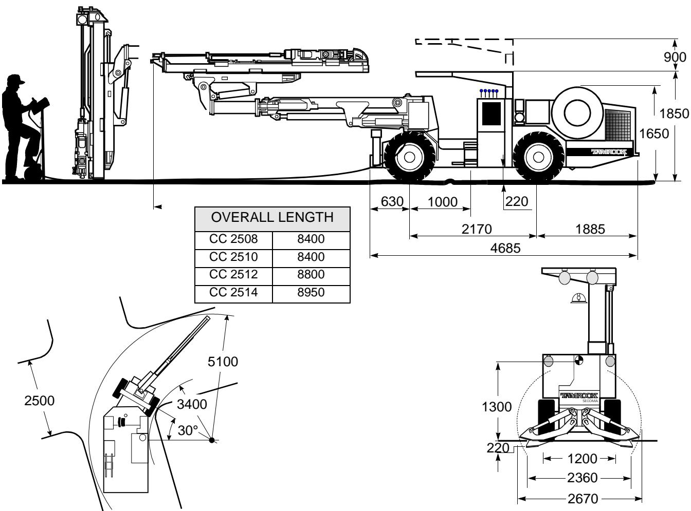
**High power compact versatile drill, four wheel drive hydraulic jumbo,
