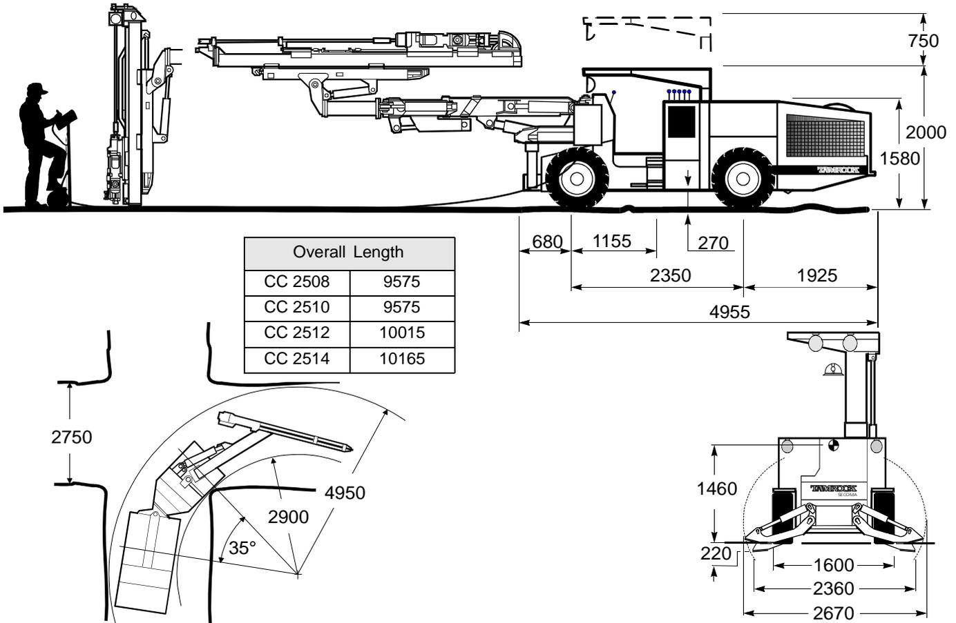
**High power compact versatile drill, four wheel drive hydraulic jumbo, for development and production in 6 to 37 m<sup>2</sup> sections.**
