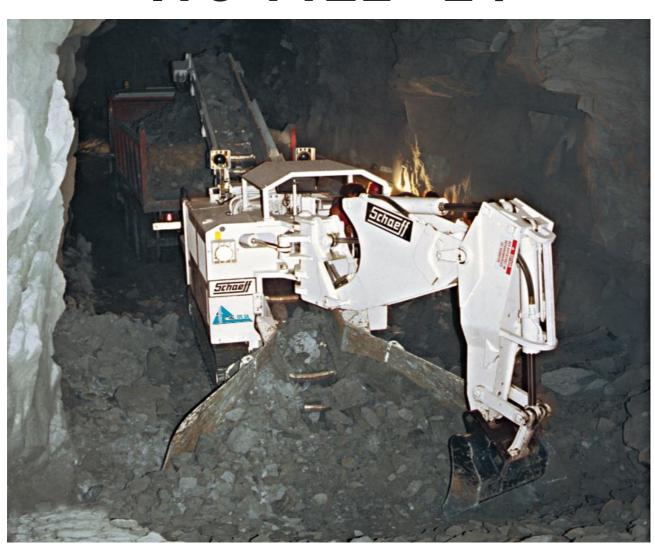
For excavation of ground and/or loading of blasted rock
