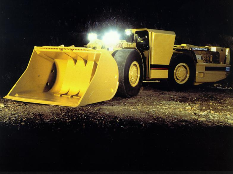
CAT® 3306C DITA (Swirl) Engine Gross Power 123 kW (165HP) Rated Load 6,500kg (14,333lbs) Operating Weight 20150kg (44,423lbs)
